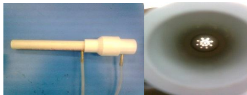
Photograph of the fabricated mouthpiece (left) and cross-section showing the laminar flow resistor (right).
