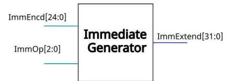
(b) Immediate Generator
