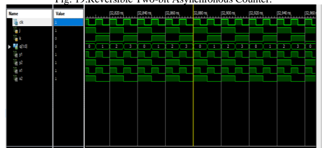
Fig. 20. Simulated output of Reversible Two-bit Asynchronous Counter.
