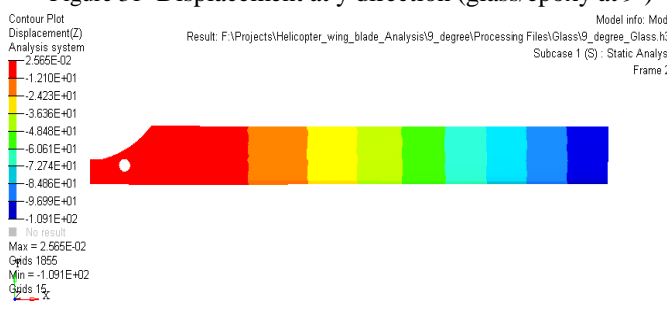
Figure 32 -Displacement at z direction (glass/epoxy at 9°)
