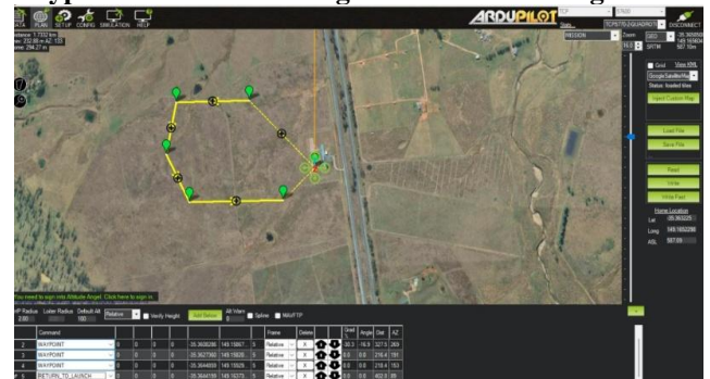
[Fig.08- Mission Planner waypoint mission setup showing five waypoints at 5 m altitude with final Return-to-Launch command uploaded to the UAV.]
