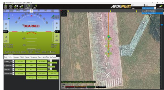
[Fig.6- Mission Planner interface showing three connected UAVs with separate telemetry ports for centralized swarm monitoring and control.]
