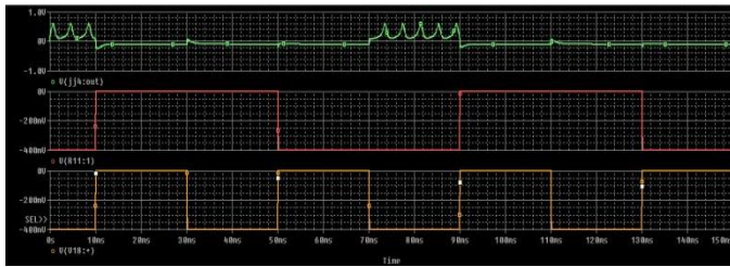
Figure 4: The Output of NOR gate.
