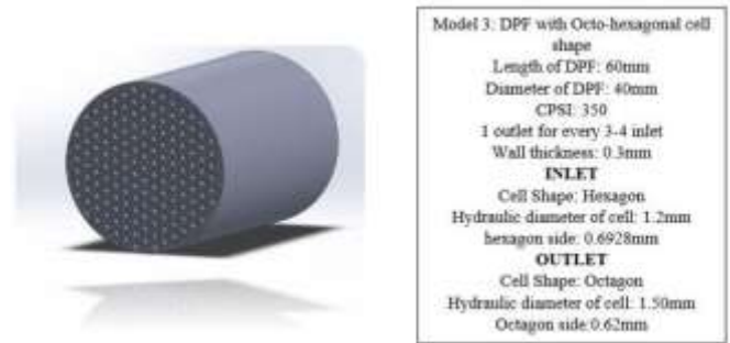
Fig. 3 Model 3: DPF with octa-hexagonal cell shape
