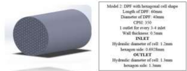
Fig. 2 Model 2: DPF with hexagonal cell shape
