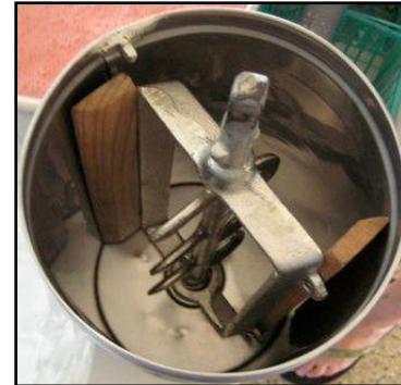
Figure1.3 Ice-cream making drum where ice-cream stirred and blended.
