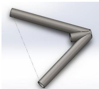
Fig. 4. 3D CAD model of Wishbone
