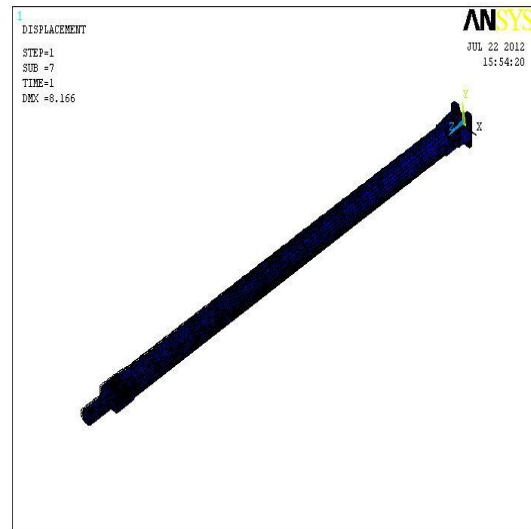
Fig 15: Kevlar/Epoxy drive shaft deformation results
