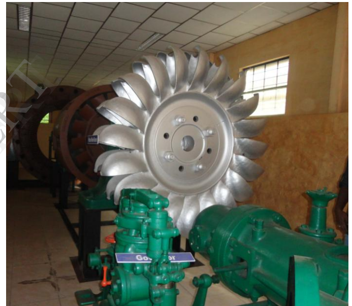
FIG 1. Pelton Runner model
