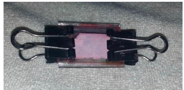
Fig.1. Manually made DSSC solar cell(Chaudhari et al,2021)
