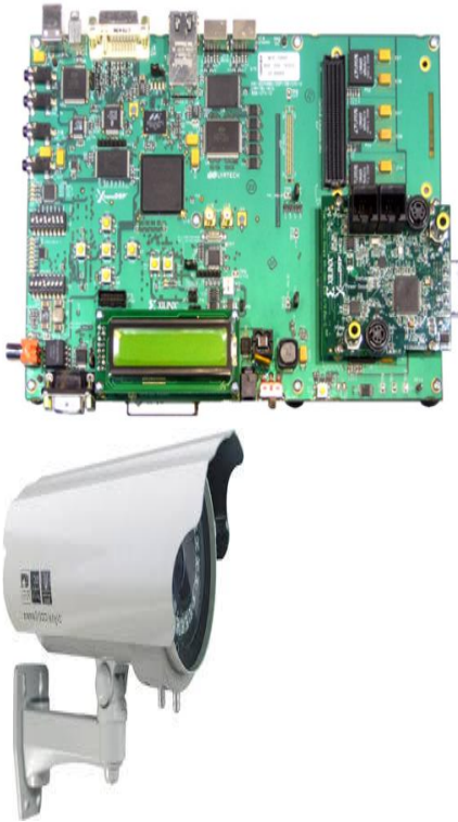
Fig.7 Spartan-3A DSP 3400 Development Platform, FMC-Video, and Camera
