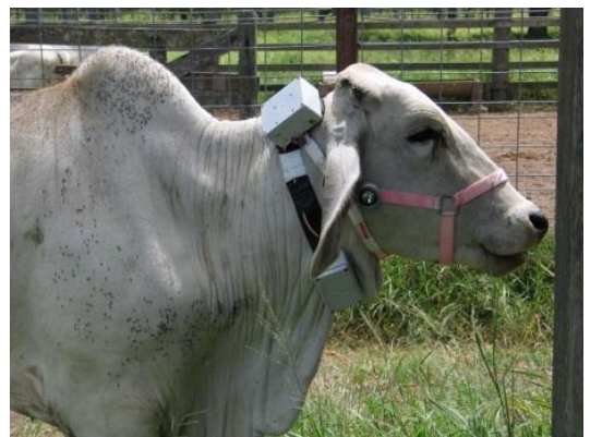
Fig: 5 Cow with Electronic Collar[7]
