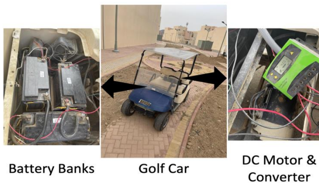
Fig. 9. Hardware implementation of the modified EV.
