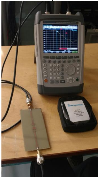
Fig. 10. Measurement of Response of the filter using VNA ZVH-8.
