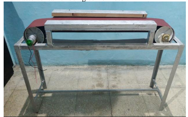
Fig. 14 Fabricated conveyor system
