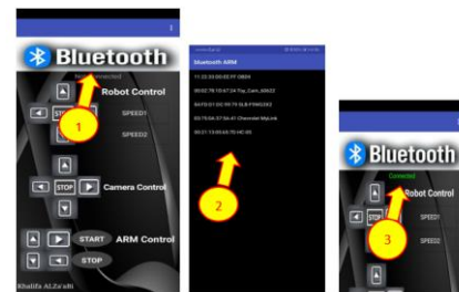
Figure (16) how to connect phone to HC-05 module
