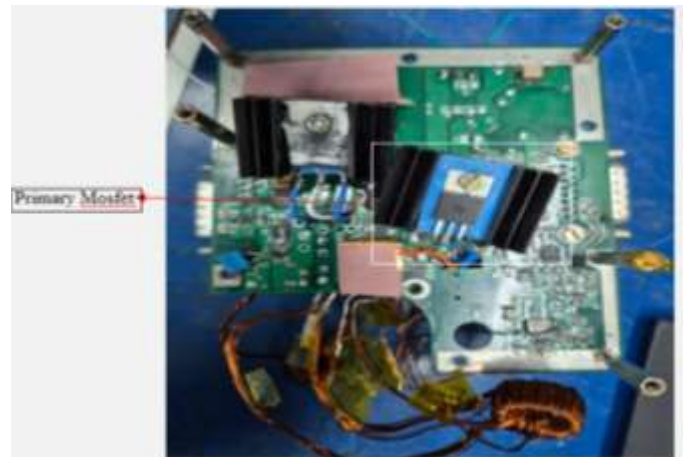
Fig. 6: PCB Bottom View of the Converter
