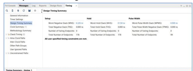
Fig. 4: Timing analysis report showing positive slack and successful timing closure.
