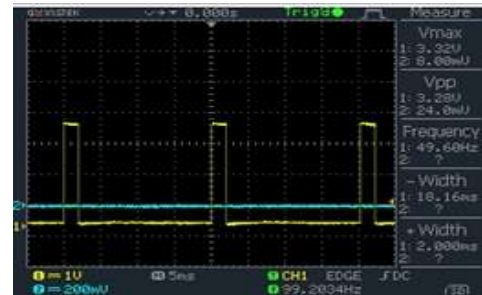
Figure 5: PWM waveform with 2ms + width
