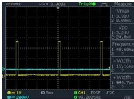
Figure 4: PWM waveform with 1ms + width
