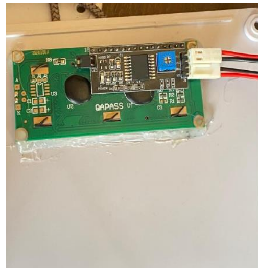
Fig 9: Assemble prototype (Inside cover showing LCD)
