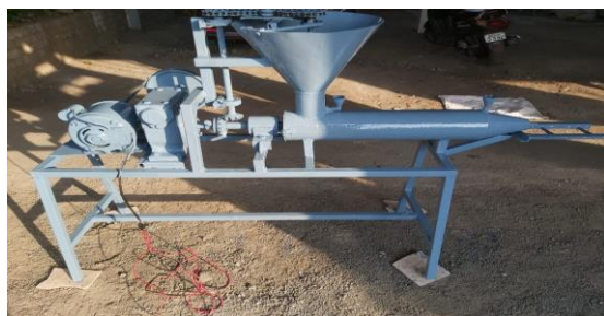
Fig-1 : The Automatic Dung Log Making Machine
