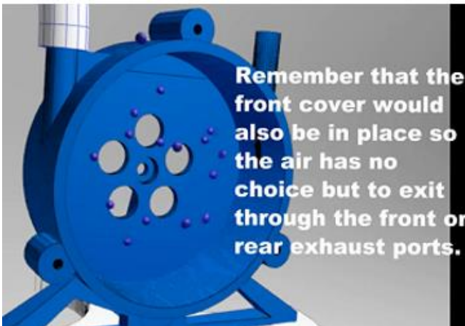
As the air molecules pass the discs they create a drag on them, this drag pulls the discs with the air, this is a basic explanation of the boundary layer effect.
