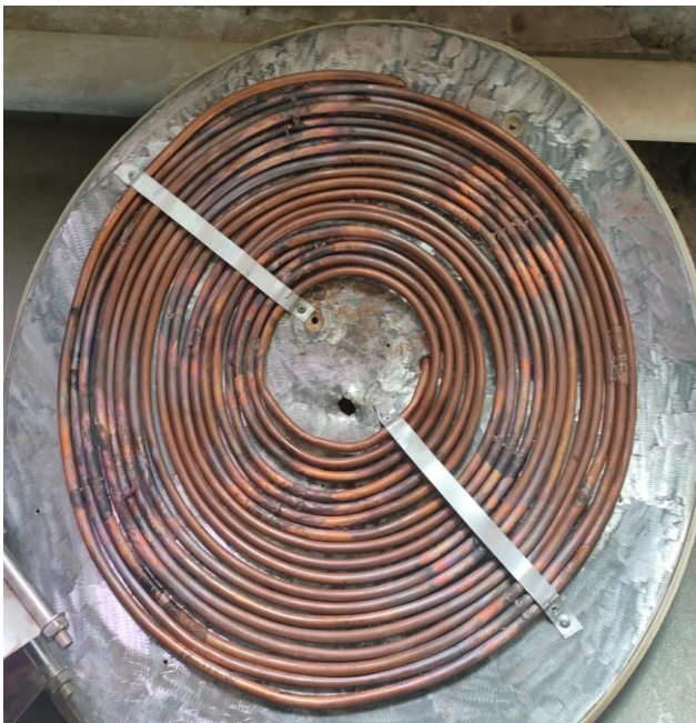
Figure 2: Copper tube collector with parabolic dish
