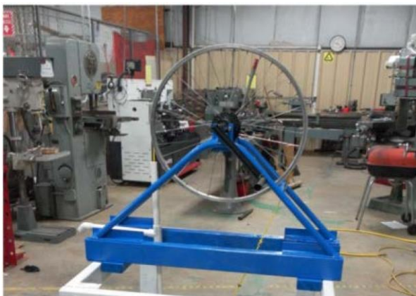
Fig 2.2 - Finalized A-Frame Support Structure
