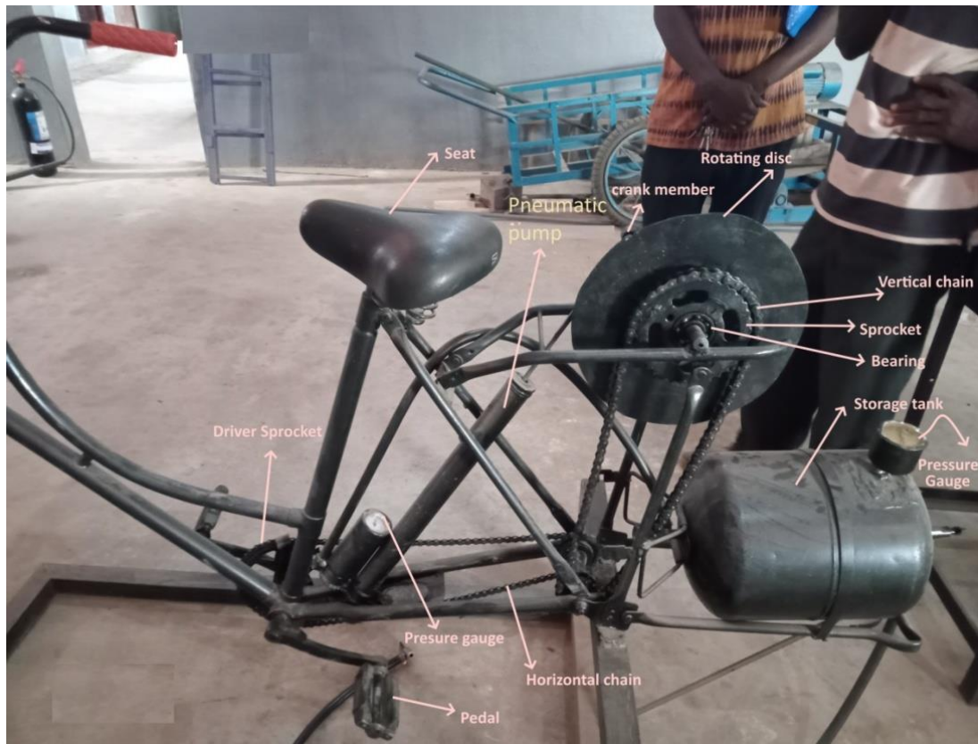
Figure 5 the Air compressor complete assembly
