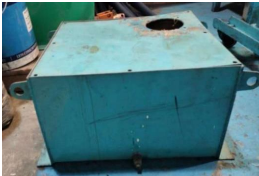
Figure 15. Hydraulic Oil Tank
