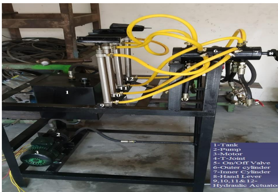
Fig 4.6 Fluid transmission paths linking the circulation hub to increment-logic manifold and on force-delivery module
