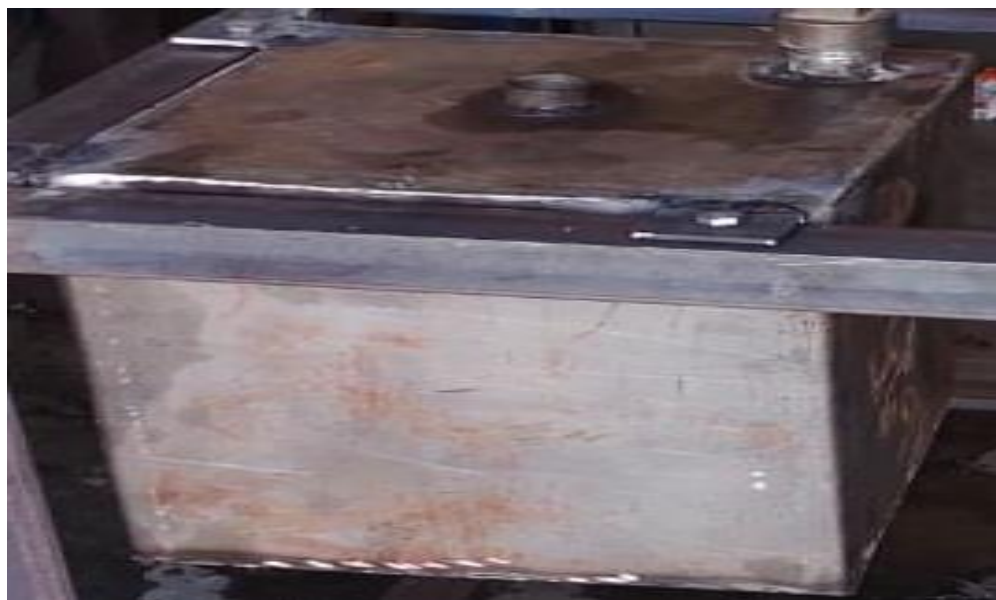
Fig 4.8 Fabricated section of hydraulic tank
