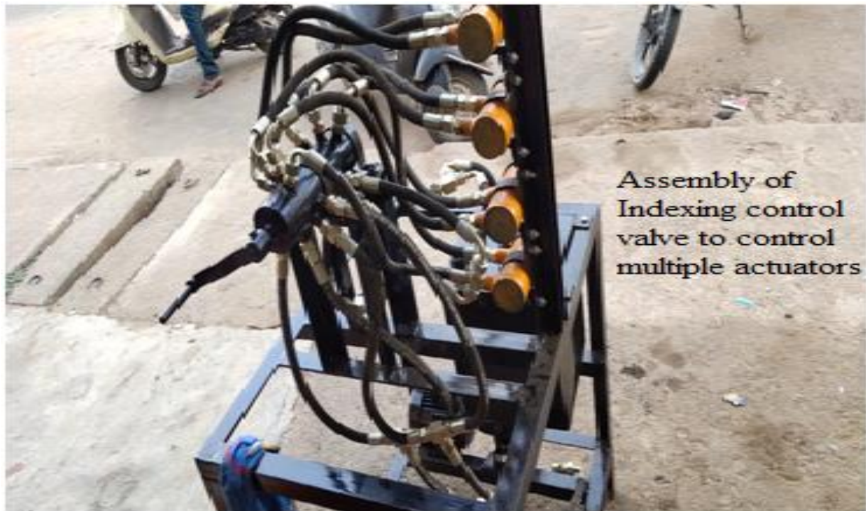
Fig 4.5 Fluid transmission paths linking circulation hub to increment-logic manifold and on force-delivery module
