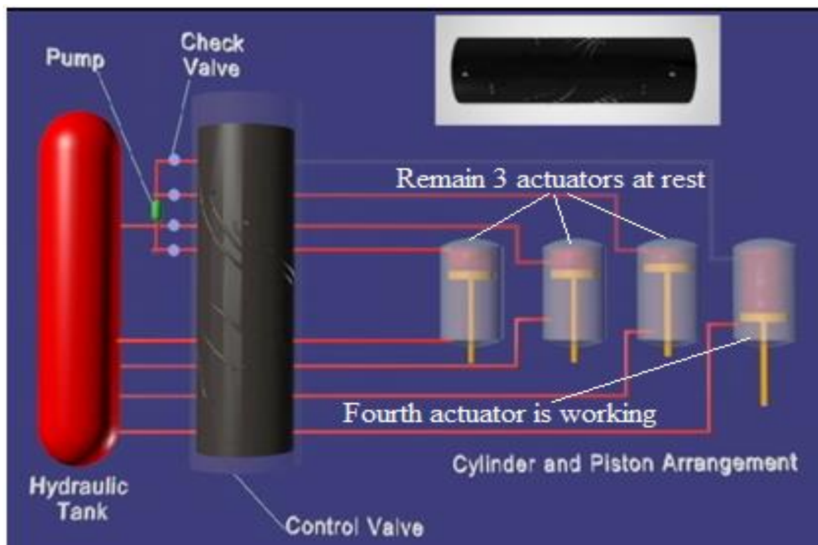
Fig 6.4 4 th actuator Operating remain 3 actuators remain at rest
