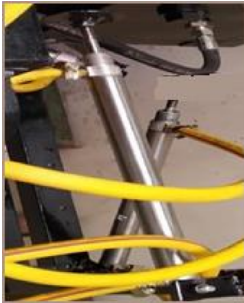
Fig 4.2 Pressurized piston-and-bore assembly
