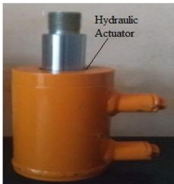
Fig 4.1 Fluid-powered motion initiator
