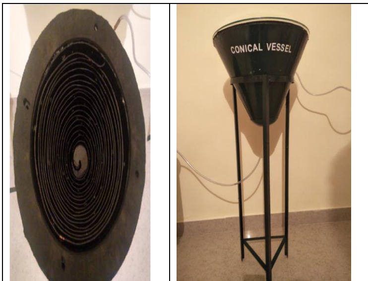
Top and Front view of Conical vessel along with spiral placing of copper tubes along the surface of the conical vessel
