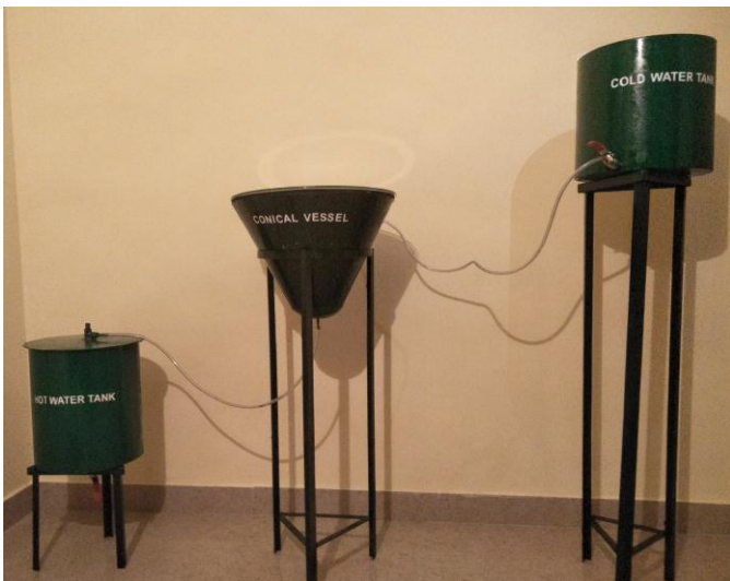
Conical Shaped Solar Water Heater Equipped with Convex Lens
