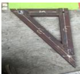
Figure 18: The triangular link cut, welded and then drilled
