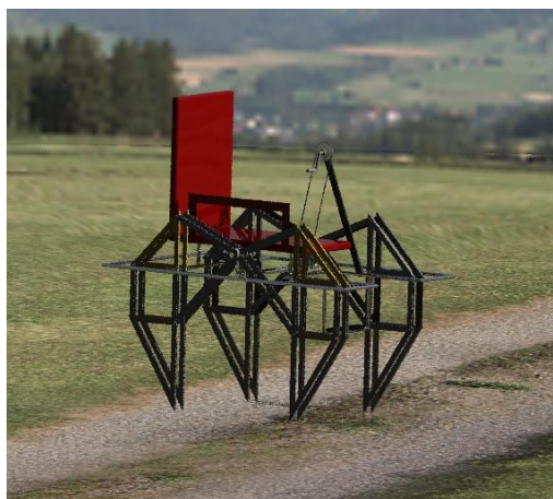
Figure 5: Autodesk Inventor rendering of the initial idea of walking chair
