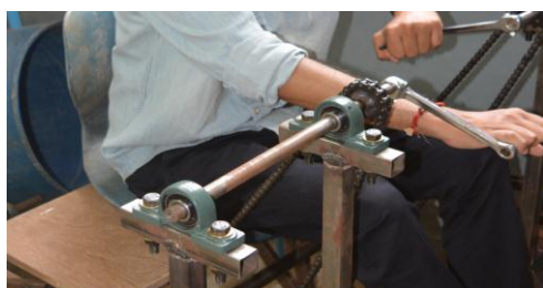
Figure 22: Image showing the drive shaft with driving sprocket and pedal
