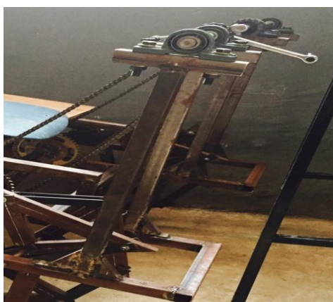
Figure 23: The T-Structures mounted on the frame
