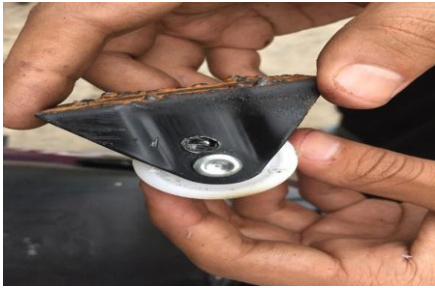
Figure 25: The fixed wheels that were attached as the foot of the system
