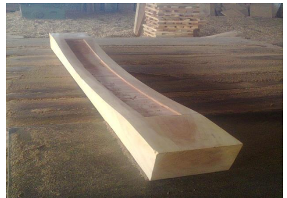
Fig5. Composite leaf spring manufacturing wooden mold.
