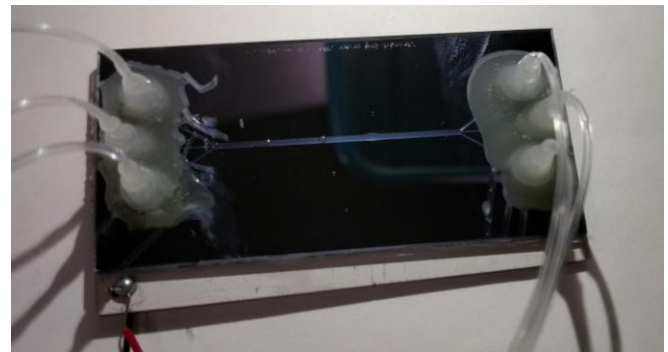
Fig. 3. Fabricated acoustic microfluidic chip with integrated piezoelectric actuator.
