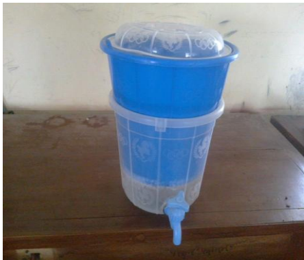
Fig. 2. An improvised filter media chamber
