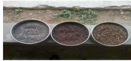
Fig. 1. Crushed nut shells (Periwinkle shells, Palm kernel shells and Coconut shells) respectively.
