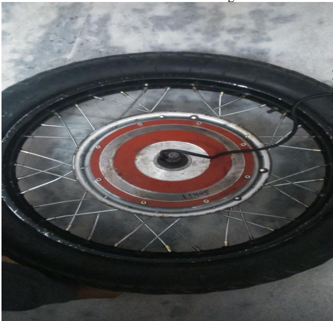
Figure 12: BLDC motor incorporated in wheel
