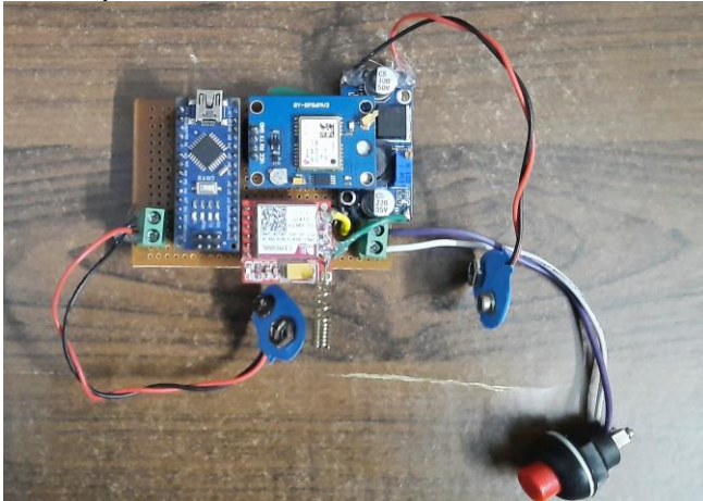
Fig:8 Hardware of transport Module
