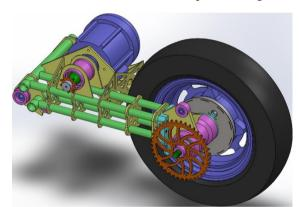
On Altair HyperWorks based on Optistruct, a static structural analysis of this subframe is performed, with boundary conditions such as fixing all DOF except rotation on pivot point, fixing vertical DOF of spring mount, motor dead weight, motor holding torque, drive train holding force, bump load, brake torque, leaning angle load, and acceleration push. The study revealed a maximum von-mises stress of 260MPa and a maximum displacement of 3.42mm. As a result, the safety factor is 1.35.
