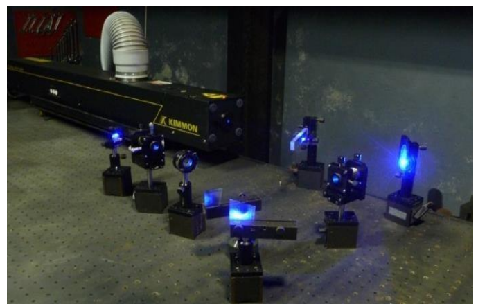
Fig. 5 Transfer hologram set up using He Cd laser
