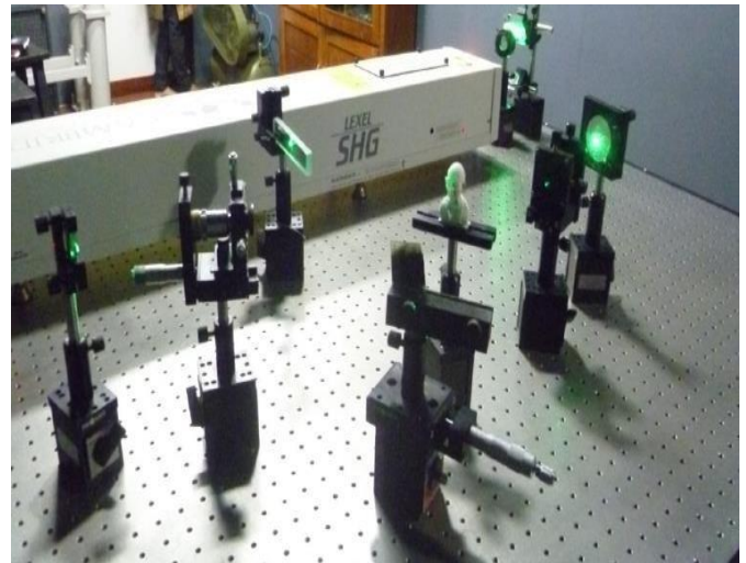
Fig.4 Master hologram set up using Argon ion laser
