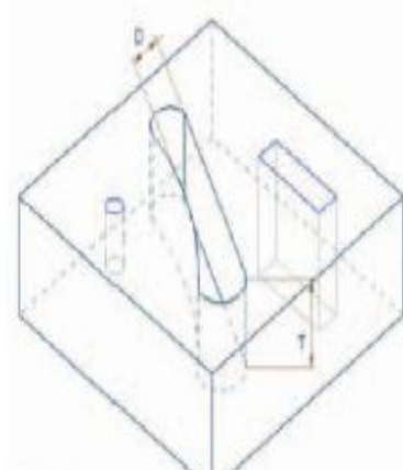
Fig. 12: Typical concave manufacturing features in mold. [5]
