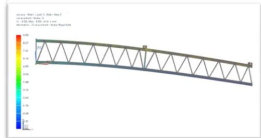
Fig 1.12 Deflection of horizontal boom
