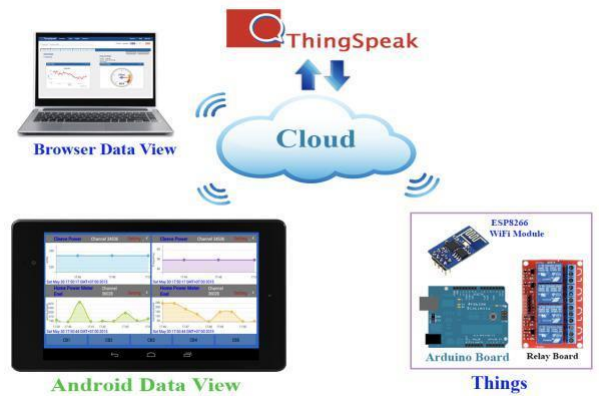
Figure 2. Working of a ThingSpeak cloud
