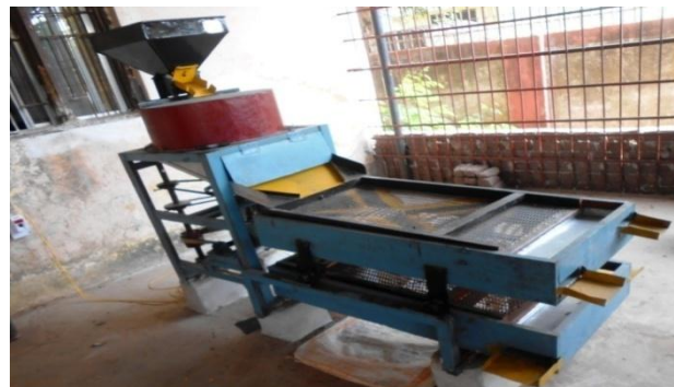
Fig. 9 Isometric view and fabrication of chironji decorticator machine.
