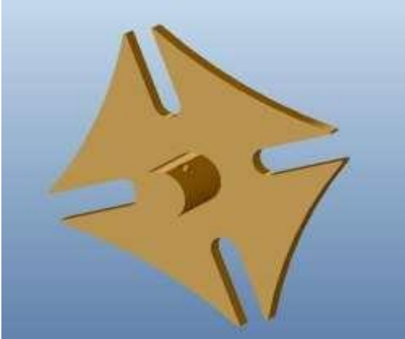
Figure 2: Traditional four-slot Geneva wheel
