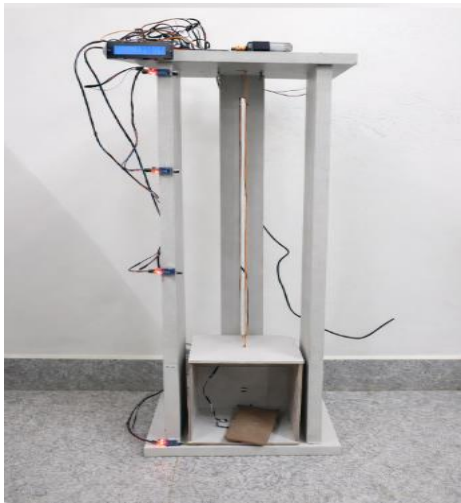
Fig 5: The hardware of prototype elevator control system controlled from the Bluetooth
