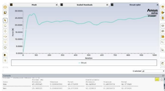
Fig 7b: Results of CFD Analysis of EDF
