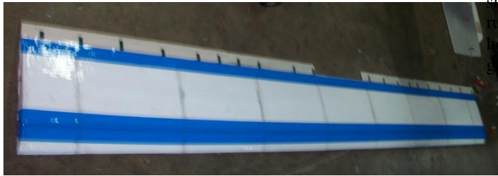
Fig 3: The final finished wing using epller 387 airfoil
