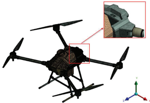
Fig. 16. Mesh of the drone
