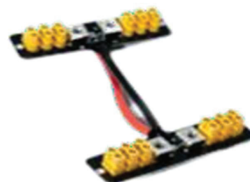
Fig. 11. Power Distribution Board
