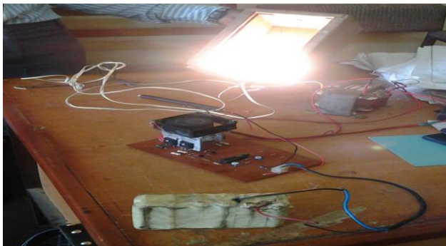
Fig-8 Performance evaluation of the output of the constructed 500watts PWM DC/AC 220V Power Inverter
