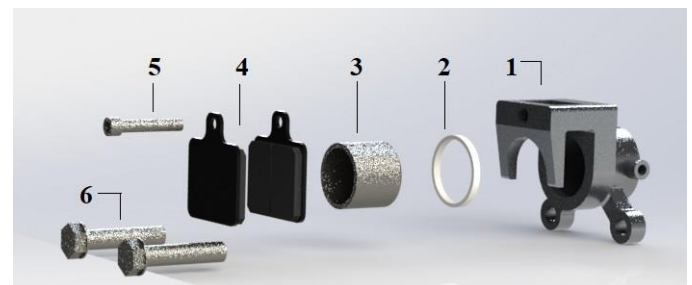
Fig. 11. Rendered image of the Brake Caliper Assembly (1) Caliper body, (2) Retraction Seal, (3) Brake piston, (4) Brake Pads, (5) Pad Pins, (6) Floating pins
