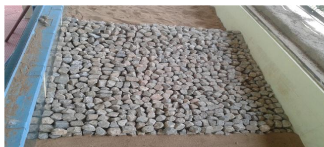
Figure (b) Top view of the seawall model before running.
