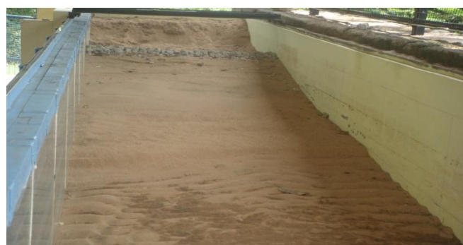
Figure (c) View of model at 5 th day cycle, good beach formation can be seen.
