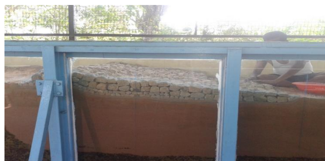
Figure (a) Side view of the seawall model before running.
